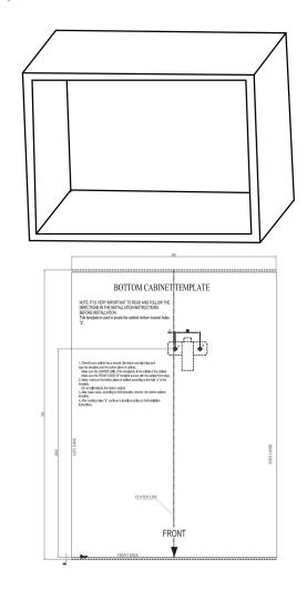
2. Make the marks on the bottom plane of cabinet according to marks "a" of the template.
