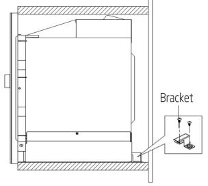
2. Open the door, fix the oven to the cabinet with Screw B through the installation hole. Then fix the trim-kit plastic cover to the installation hole.
