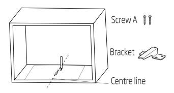
3. Remove the bottom cabinet template and fix the bracket with screw A.
